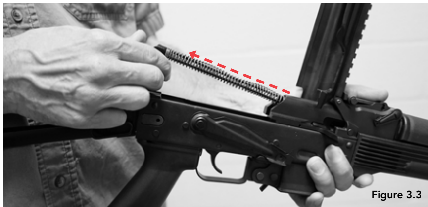
Figure 3.3 — Detaching The Recoil Spring Guide Assembly
